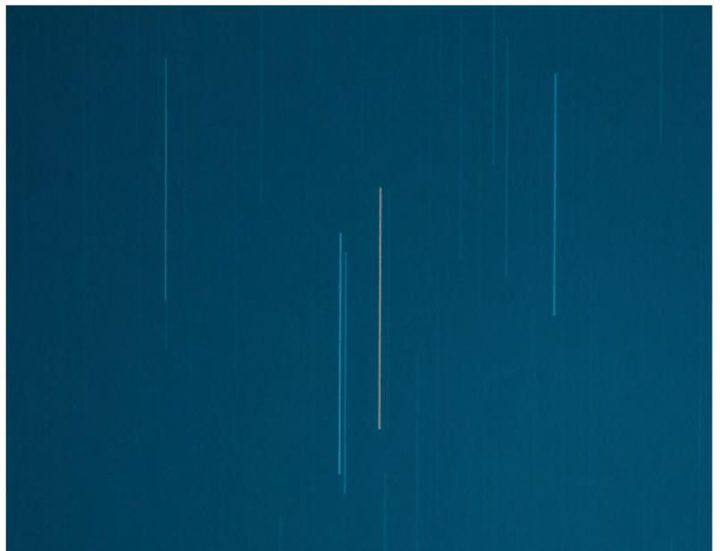
**Image 12 - Another single 3.5-minute exposure at 300-mm captured with the mount purposely misaligned by 60 degrees. The straight, true star trails offer proof of exceptional tracking accuracy.**
