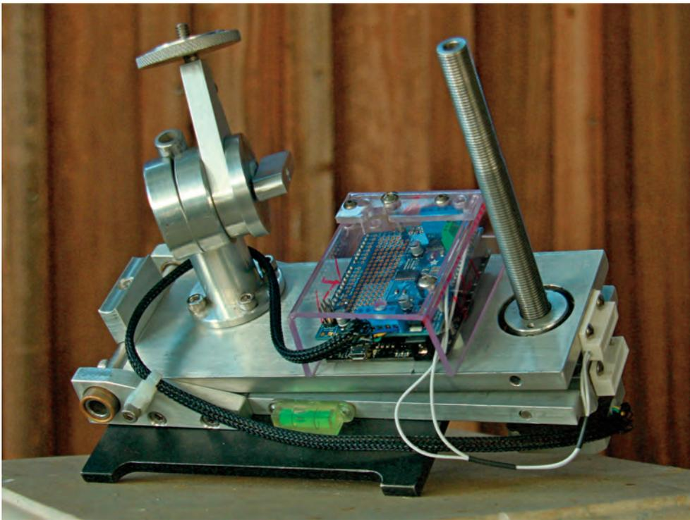
Image 2 - The StarSync camera tracker uses a leadscrew drive system as is typical of barn door-style trackers. The leadscrew is driven by a stepper motor. As it rotates, it moves a drive nut along its length. The drive nut in turn moves the upper plate, and the camera mounted on it, in the desired arc.
