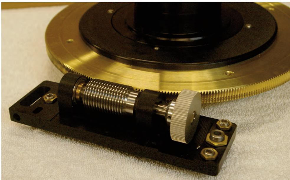
**Image 1 - A high-precision stainless-steel worm screw (foreground) and bronze worm wheel (background) by Mathis Instruments machined to an accuracy of  $\pm 0.0001$  inches in residual run-out and thread lead error for native tracking accuracy of  $\sim 5.0$ -arc seconds peak-to-peak error.**
