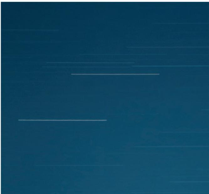
**Image 11 - TA single 3.5-minute exposure at 300-mm, cropped to show detail, captured with the Lightrack II purposely misaligned by 60 degrees to show tracking error. Resolution of the imaging system was 2.95 arc seconds per pixel, so the images demonstrate absolutely minimal error.**
